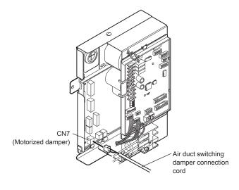
(4) Remove the cord bush from the terminal block cover. Pass the air duct switching damper connection cord through the cord bush. Fix the cord bush on the cord (black) section.
