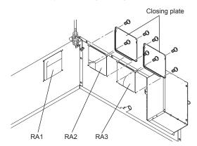
(2) Cover the RA1 opening using a removed closing plate and four screws (4-6 mm). (Screw tightening torque: 1.2 to 1.5 N·m)
